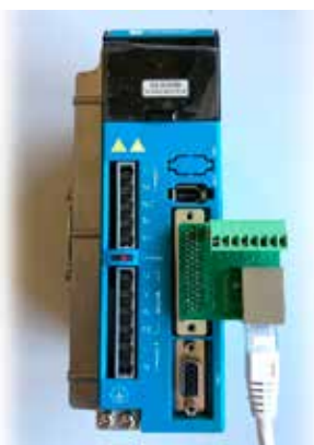
Examples for using RJ45-adapters on Leadshine Motordrivers
