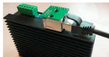
Examples for using RJ45-adapters on Leadshine Motordrivers
